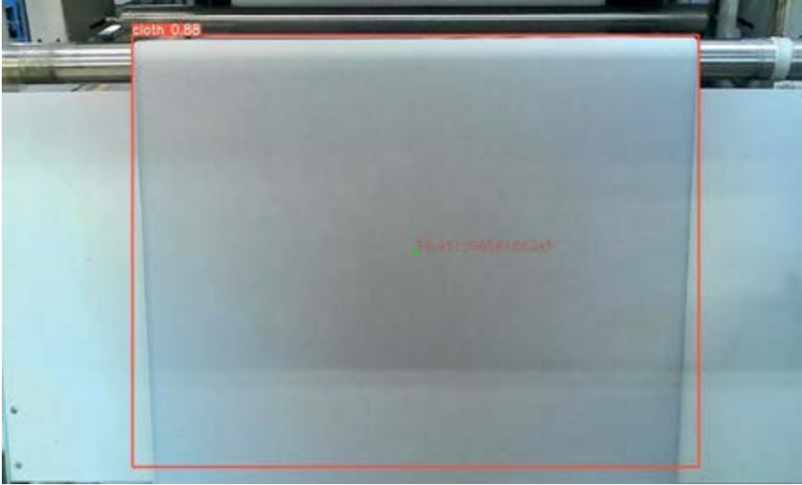
Figure 10. Predicted width at 59.95inc. of fabric.
