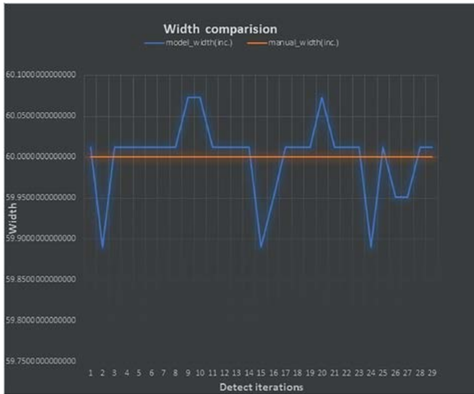
Figure 12. Graphical representation of predicted width and manually measured width.
