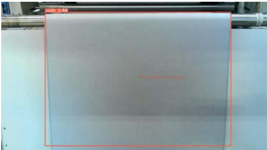
Figure 11. Predicted width at 60.07inc. of fabric.
