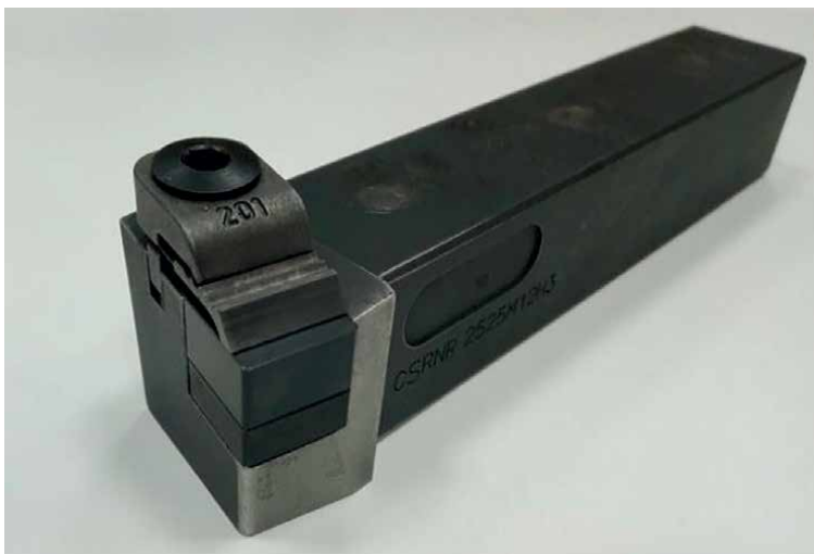
Figure 1. Appearance of cutting board holder CSRNR 25 × 25 M12H3 from the company HERTEL (owned by the faculty of mechanical engineering in Skopje) [1].
