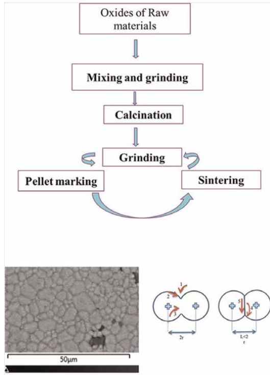
Figure 2. A flow chart provided for developing GdCa_2Cu_3O_8 using a solid-state reaction method and SEM micrograph of ceramic [11, 12].
