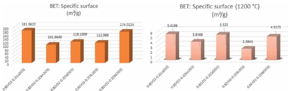
Figure 9. BET specific surface area analyzed for the five specimens. Left: As obtained 0.8ZrO 2 -0.2(Ln 2 O 3 ); right: 0.8ZrO 2 -0.2(Ln 2 O 3 ) heat-treated at 1200°C, where Ln = La, Nd, Yb, Sm.
