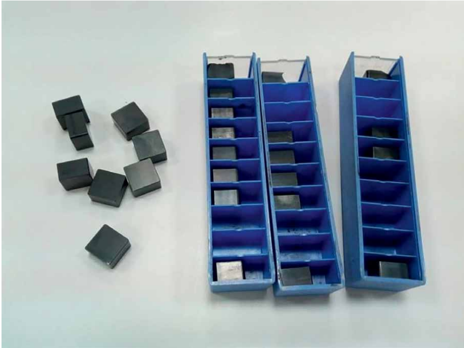
Figure 5. Appearance of cutting plates SNGN 120708-120,712-120,716 from mixed ceramics MC 2 ( \text{Al}_2\text{O}_3 + \text{TiC} ) from the company HERTEL [1].
