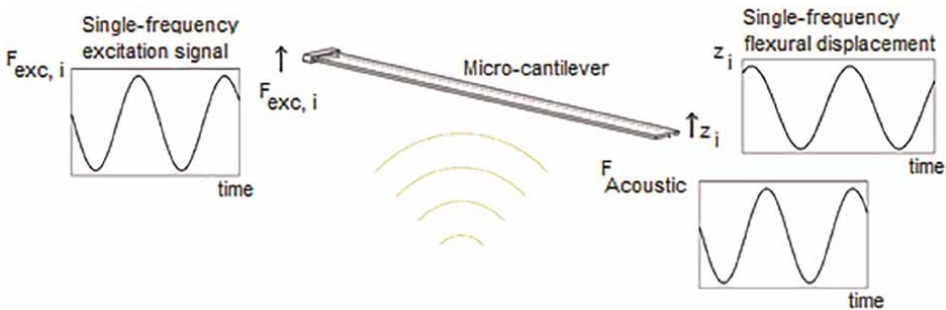
Figure 1. A schematic representation for single-frequency flexural deflections of the resonant micro-cantilever under dynamic acoustic forces for the first two eigenmodes under monomodal operations.
