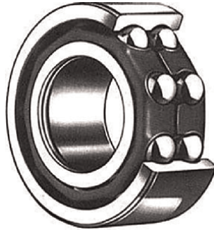
Figure 4. Cut-away view of a double row of ball rollers in a bearing assembly.
