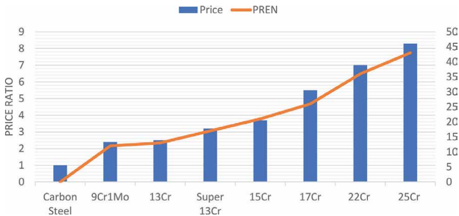
Figure 3. Overall price ratio comparison between different grades of CRA and carbon steel, along with their corresponding Pitting Resistance Equivalent numbers (PREN) [9].
