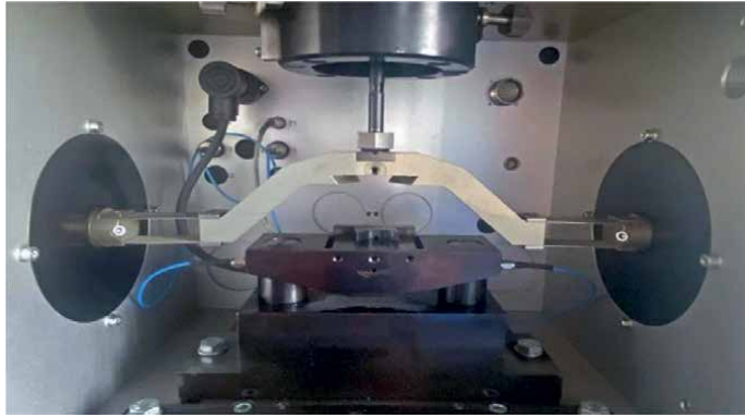
Figure 10. Modified bench testing for piston skirt coatings to simulate the relative motion between a piston and a liner of typical engine operating conditions.
