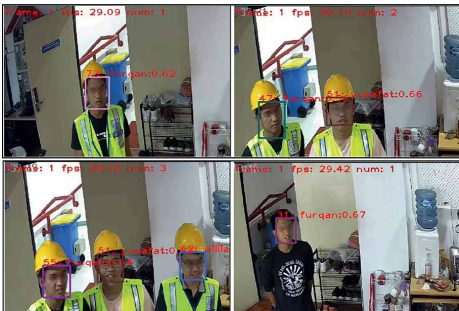
Figure 8. Face detection accuracy results in mining simulation.
