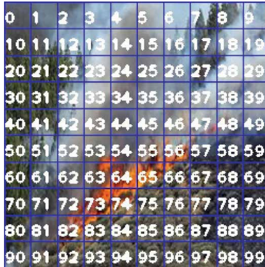
Figure 3. Example of an image divided into 100 small parts (sub-images).
