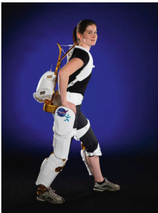
Figure 7. The NASA X1 Robotic Exoskeleton for resistive exercise and mobility augmentation, with 4 motorized joints and 10 degrees of freedom (Credit NASA).
