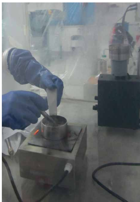
Figure 8. Oxygen-free glove-box to solids drying and sample splitting under nitrogen gas atmosphere.
