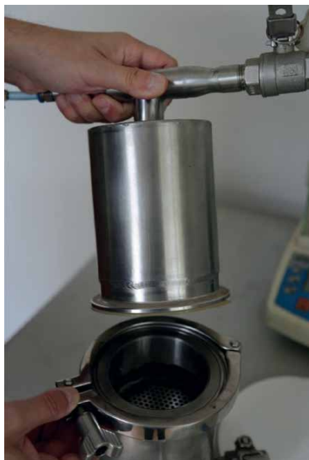
Figure 7. Slurry filtering chamber. To remove the air from the chamber, the valves allow injecting nitrogen gas as well as dissolved oxygen-free water towards the end of the filtration stage for washing purposes.
