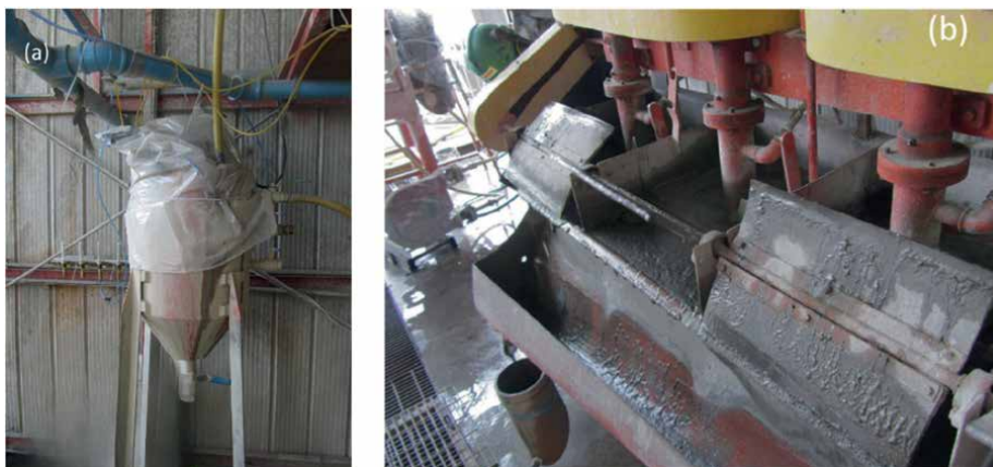
Figure 4. Pictures of the pilot plant used in the project to evaluate the impact of oxygen concentration when dosing the isobutyl xanthate collector (a) oxygen concentration tuning reactor wrapped in plastic, (b) rougher bank.
