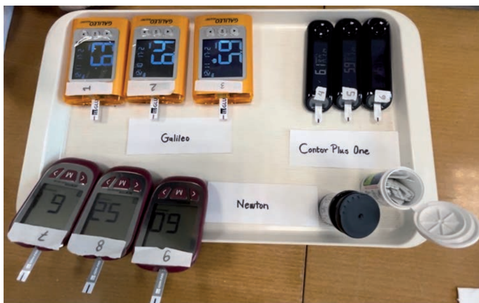
Figure 2. The three GSS used: Contour Plus One (top right), Newton GDH-FAD (bottom), Galileo Glu/Ket (top left). All nine glucometers showing different values of cPG in mmol/L estimated from the same drop of blood collected from a single finger-prick.
