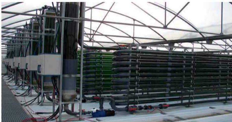
Figure 1. The University of Almeria's department of chemical engineering created a vertical tubular serpentine photo bioreactor (Spain) [47].
