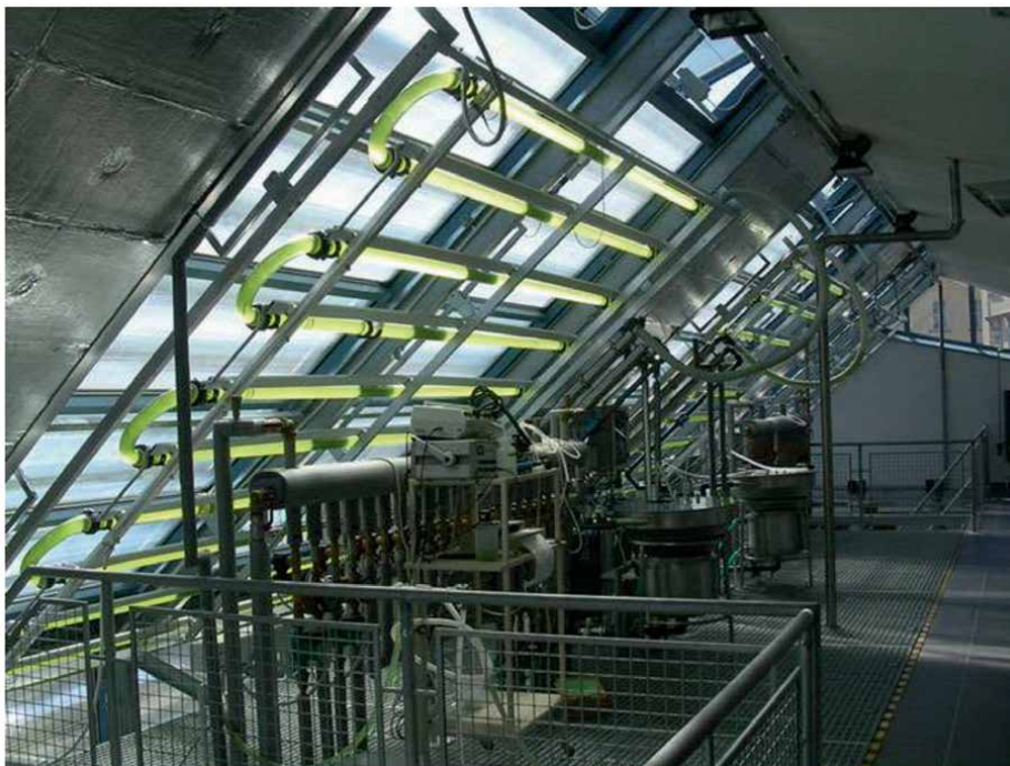
Figure 3. A linear Fresnel lens-based solar concentrator-based tubular serpentine photo bioreactor was created at the University of South Bohemia's center for biotechnology in Nové Hrády (Czech Republic).
