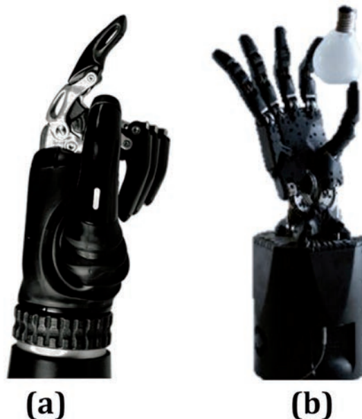
Figure 10. (a) Multifunctional prosthetic hands. Modified from the public domain image [43] (b) Shadow Dextrous Hand is considered to be the most dextrous humanoid Robot hand. Source: Ref. [44].
