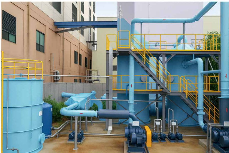
Figure 23. Pilot plant for CaCO 3 construction material production (Daewoo Engineering and Construction Co., CO 2 treating capacity 1 ton/day).
