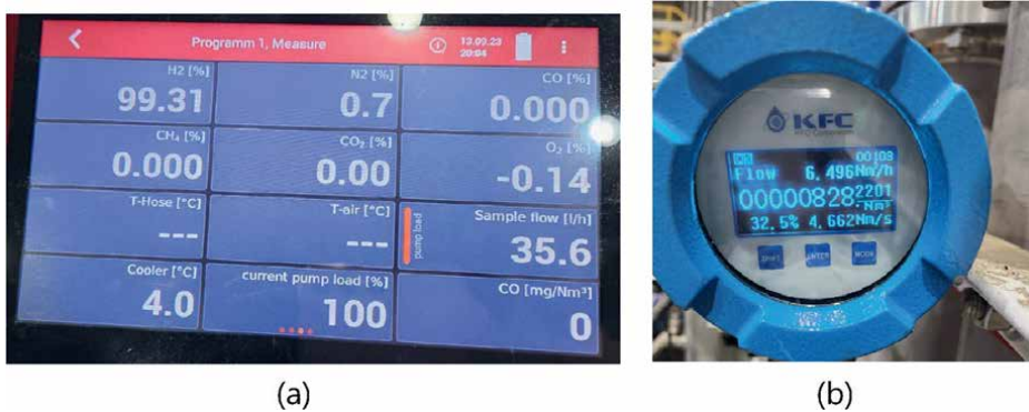
Figure 14. Operation results of PSA process in pilot-scale plant (a) Pressure trends of H 2 in PSA tower (b) H 2 gas flow rate measured.
