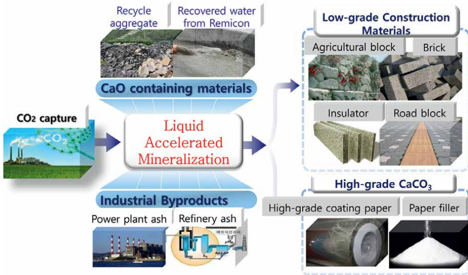
Figure 22. Concept of CO 2 mineralization to utilize captured CO 2 .
