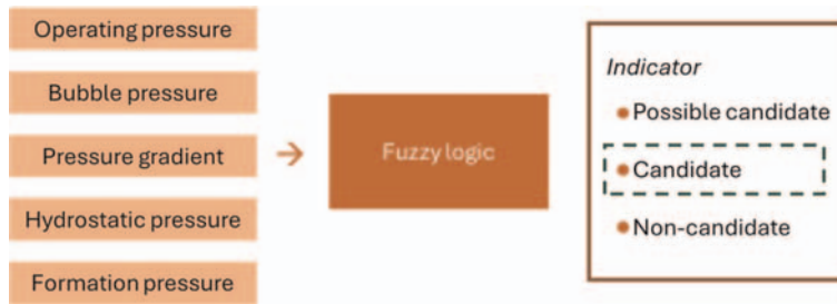
Figure 2. Fuzzy logic system for categorizing oil wells.
