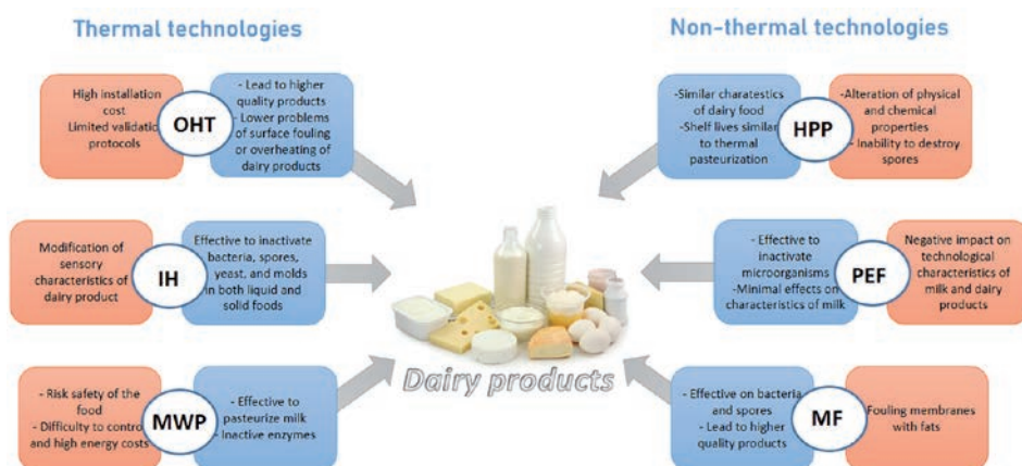
Figure 1. Main benefits (blue box) and drawbacks (orange box) of novel thermal and nonthermal processing technologies in the dairy industry. Abbreviations: OHT: ohmic heating technology; IH: infrared heating, MWP: microwave processing; HPP: high-pressure processing, PEF: pulsed electric field; MF: membrane filtration.
