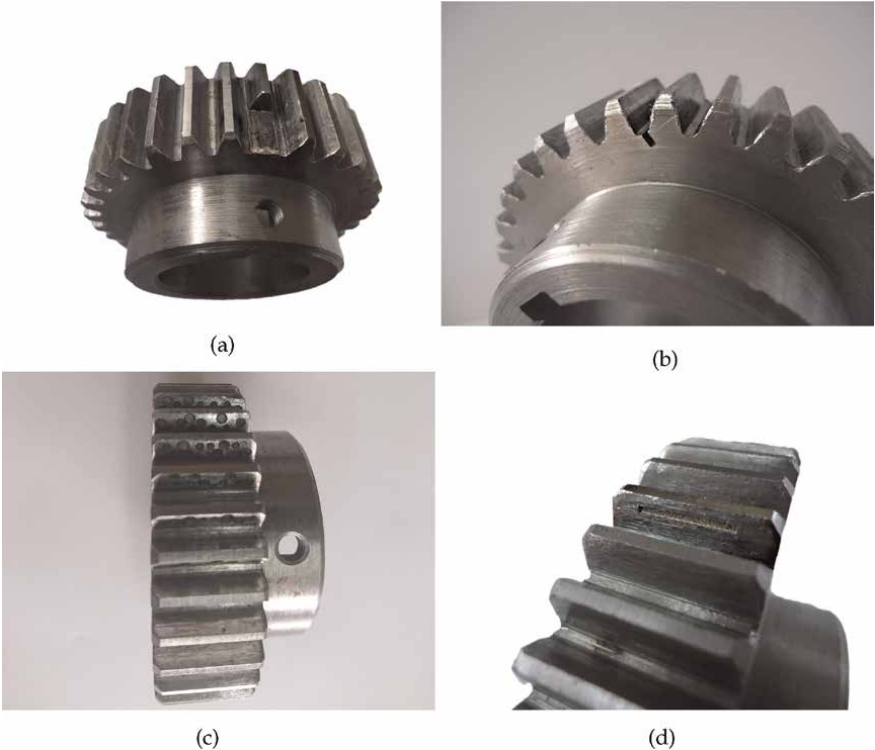
Figure 3. Simulated failure types in gear. (a) Break, (b) Crack, (c) Pitting, and (d) Scuffing.
