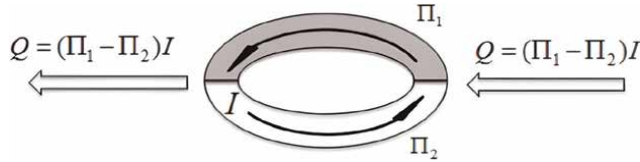
Figure 1. Cooling or heating at the junctions of two materials occur because of the different Peltier coefficients of the two materials, which can be used as thermoelectric refrigerators or heat pumps.
