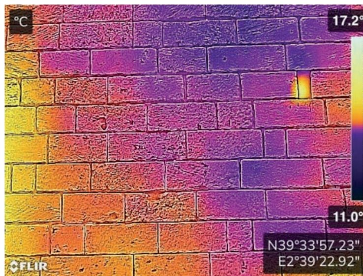
Figure 12. Thermogram of the image in Figure 11, highlighting the material differences (photo by the author).
