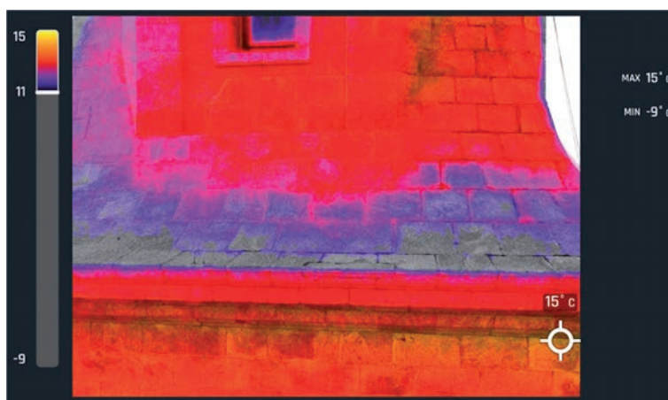
Figure 29. Junction between the original Roman section and the lantern added in the eighteenth century, highlighting the area with the highest recorded temperature (photo by the author).
