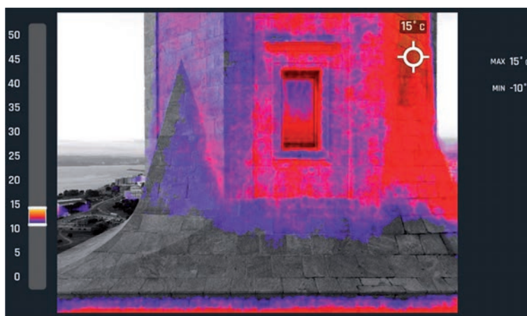
Figure 30. Thermogram analyzing the lantern atop the tower, marking the point of maximum temperature (photo by the author).
