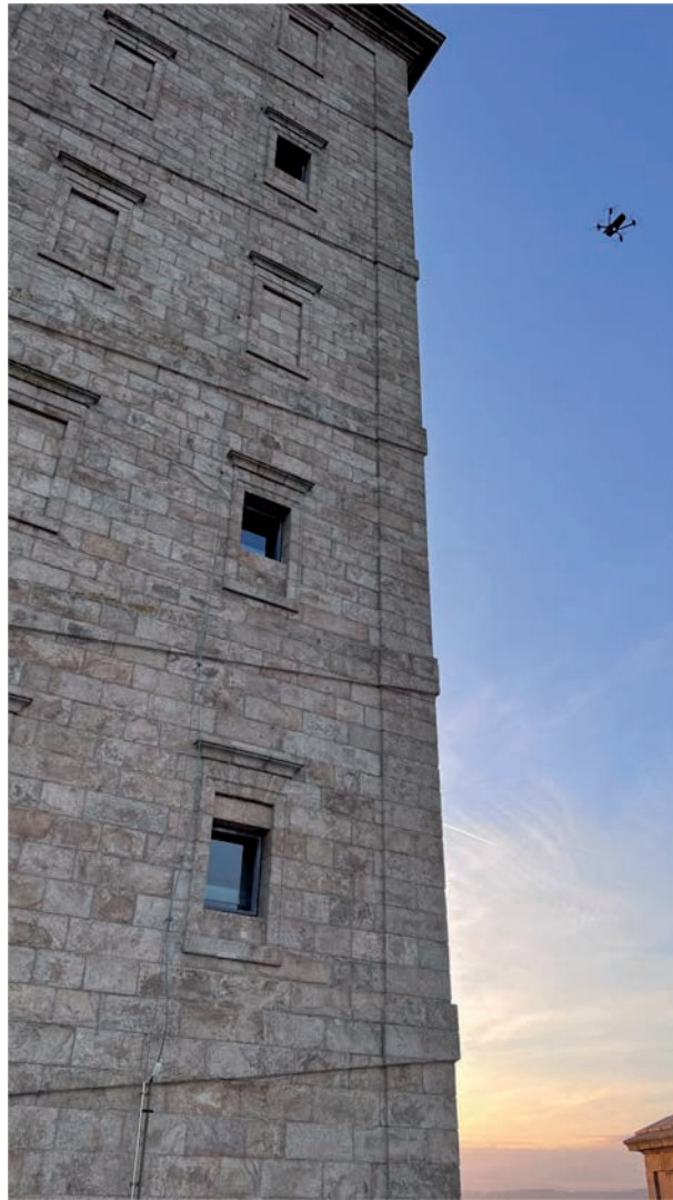
Figure 28. Drone flying alongside the Tower of Hercules to capture photographs and thermograms (photo by the author).
