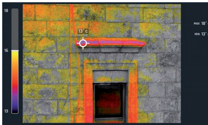
Figure 31. Thermogram captured by the drone to analyze the window of the first-level chamber on the northern facade, indicating the point of minimum temperature (photo by the author).
