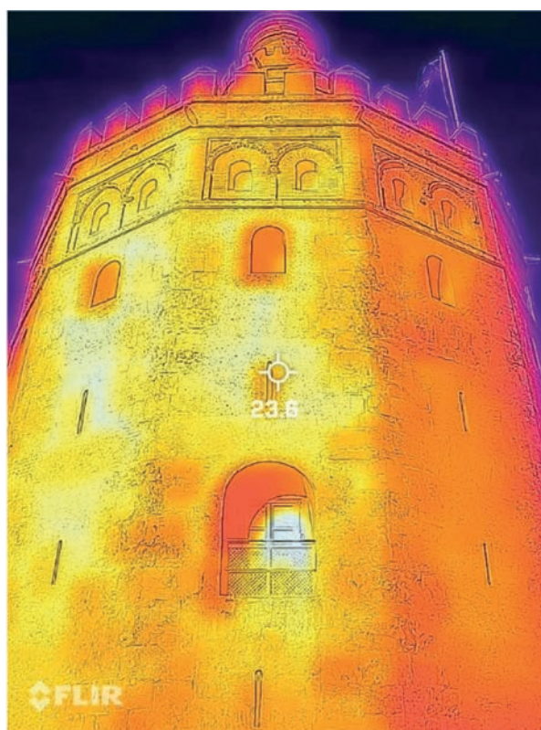
Figure 6. Thermogram of the image in Figure 5, clearly showing the different materials used in construction (photo by the author).
