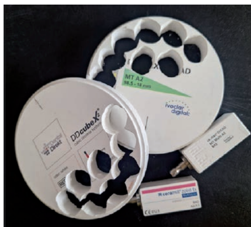
Figure 1. Zirconia blocks and disks in the pre-sintered state after milling the dental restorations.
