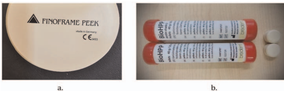
Figure 2. Presentation of HPP materials: (a) PEEK blank and (b) reinforced PEEK pellets.
