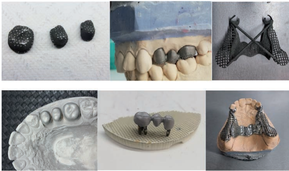
Figure 6. SLM metallic infrastructures, before and after finishing.
