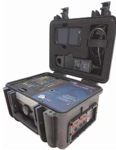
Figure 5. Integration of OMTDR into a portable electrical troubleshooting test tool, the Electrical Ground Support Equipment (E-GSE) TC50 e-tool.
