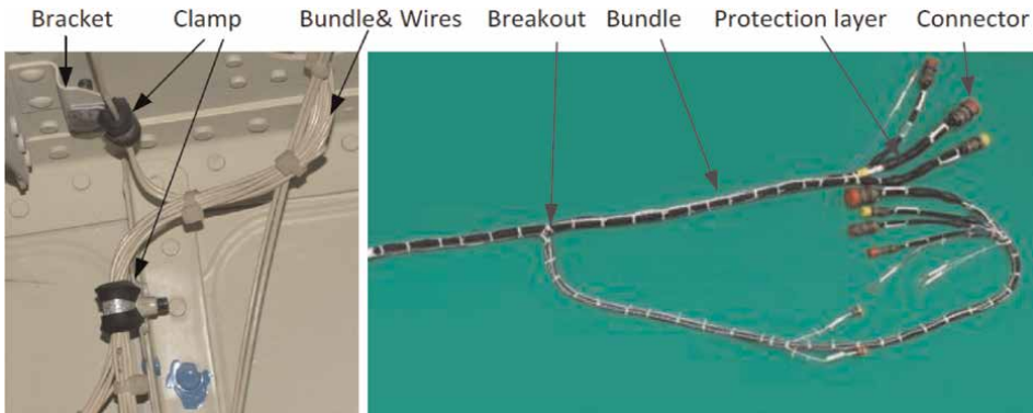
Figure 1. EWIS in an aircraft (left) and an EWIS with an independent view (right) [6].
