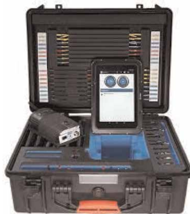
Figure 6. Integration of MCTDR into a portable tool, Aero Smart-R kit.
