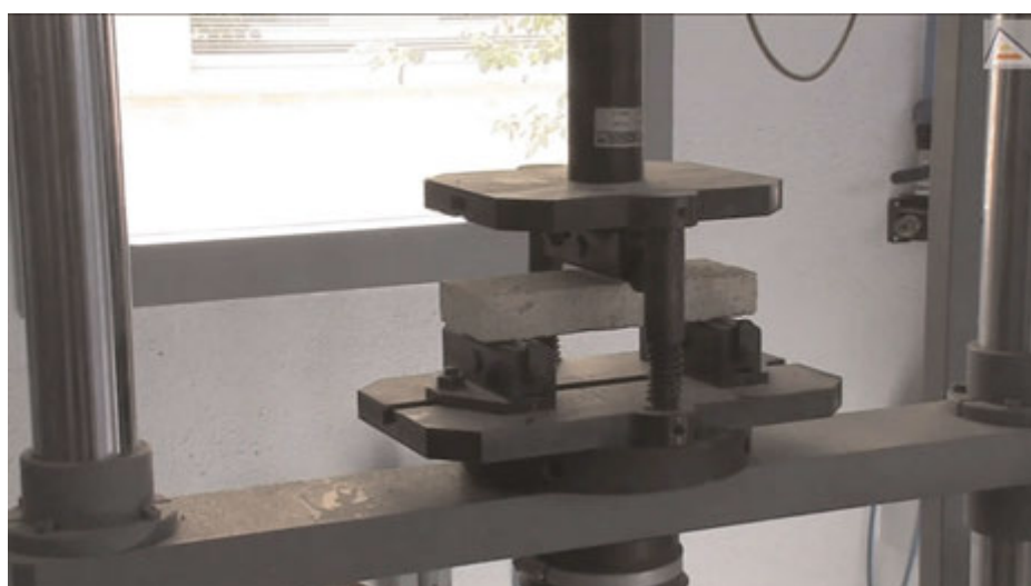
Figure 17. Test to determine the flexural strength (graphic by Alicante University [19]).
