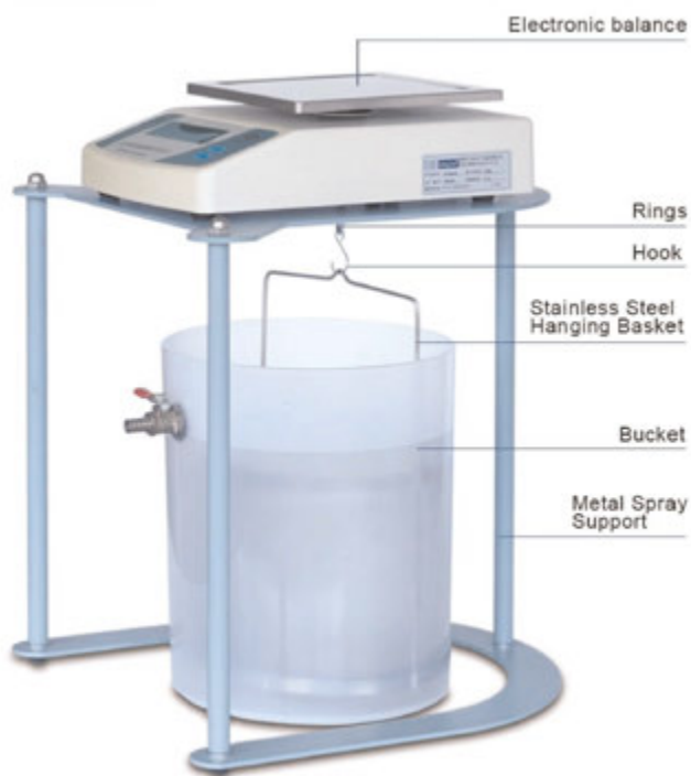
Figure 10. Balance for determining the weight of submerged rock samples (graphic by Goyojo).
