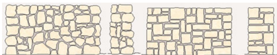
Figure 8. Masonry wall with two exposed faces, with ordinary and concerted work (graphics by Generador de Precios. Spain [6]).
