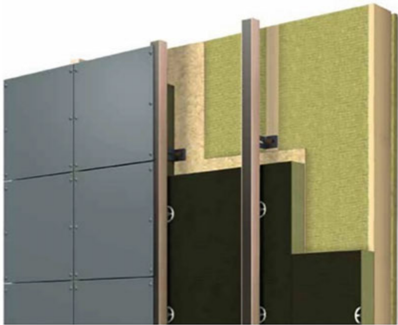
Figure 12. Three-dimensional exploded view of solution 4.
