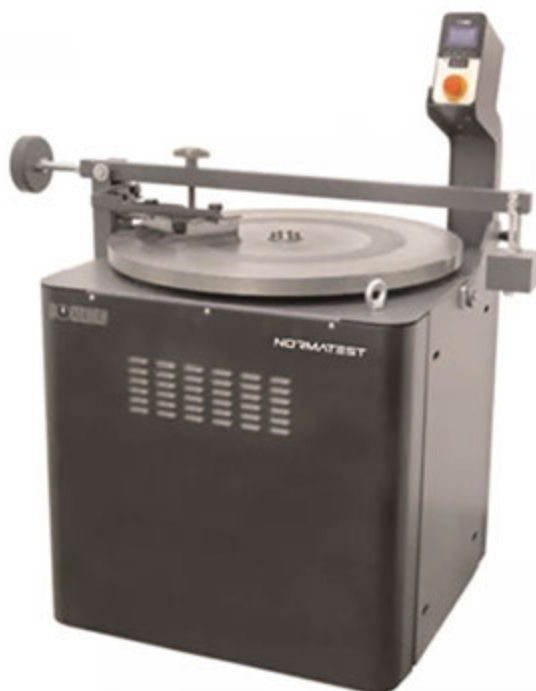
Figure 19. Device for determining the abrasion resistance of rocks used in facades (graphic by Normatest [23]).
