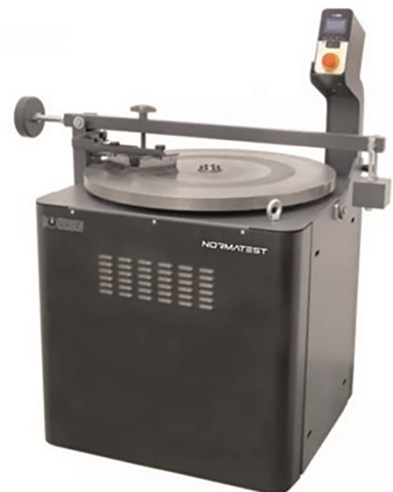
Figure 19. Device for determining the abrasion resistance of rocks used in facades (graphic by Normatest [23]).
