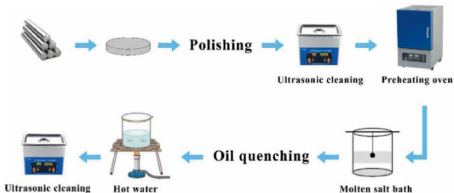
Figure 1. General scheme for the thermo-reactive deposition-diffusion (TRD) process [10].
