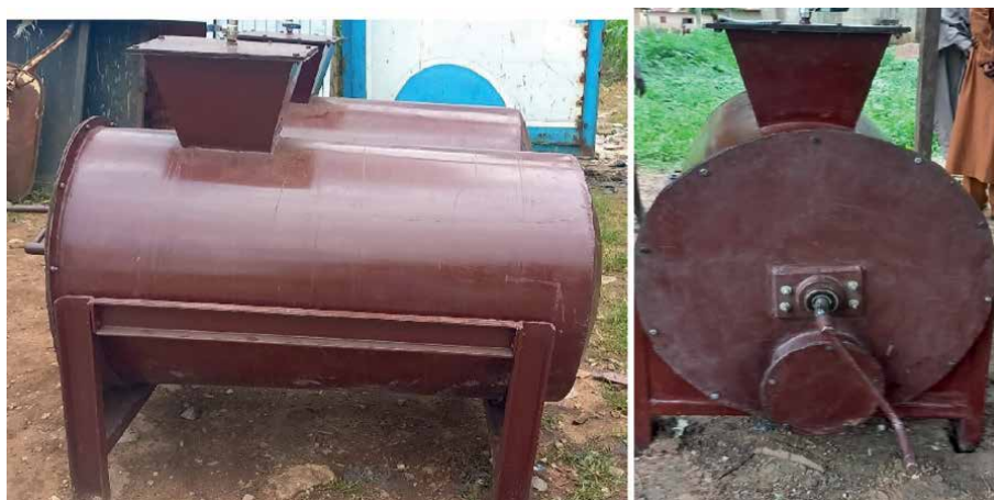
Figure 5. Locally designed and fabricated compost bio-digester used for compost production in the study.
