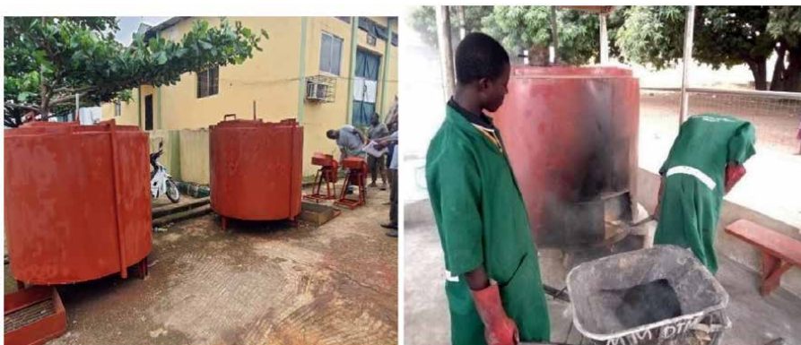
Figure 4. Locally designed and fabricated biochar kiln in use for the production of biochar at Ggbamanda production center in gidan mangoro village, Bosso LGA, Niger state.
