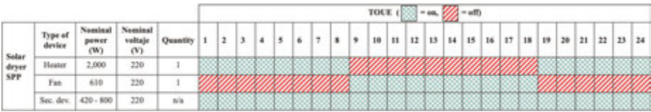
Figure 6. Results of the semi-structured survey: technical information of the SPP's electrical equipment and their TUE.
