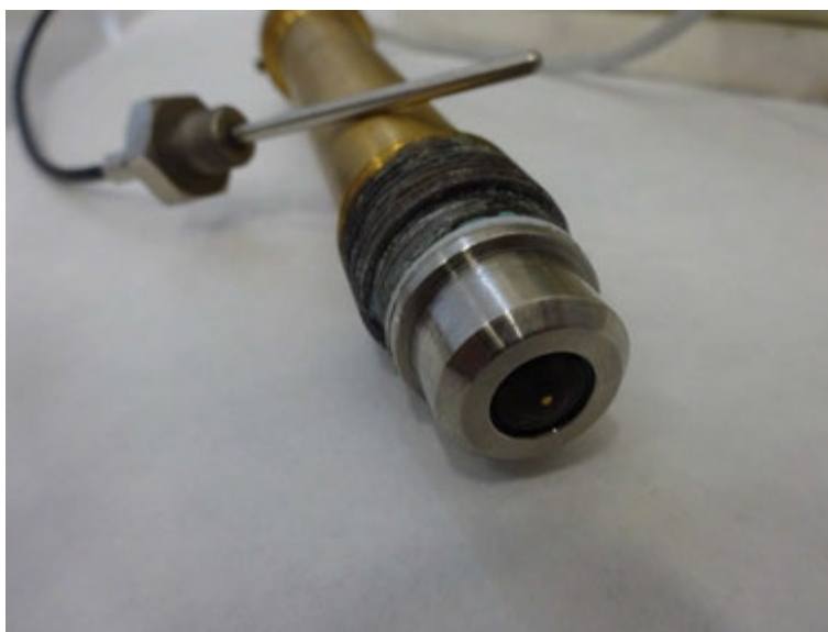
Figure 7. The hydrogen sensor with the membrane-covered platinum anode in the geometric configuration used for the measurement in primary circuit sampling channel in the NPP Dukovany. A thermometer is also visible.
