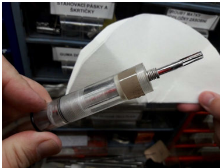
Figure 6. The inner part of the sensor, with a glass rod containing a platinum anode and a silver cathode wrapped around the glass rod.
