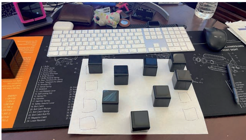
Figure 9. Illustrates the disassembly of the WowCube into individual modules and then organized in a flat plane, where it is being utilized as a modular augmented reality (AR) map. Each module is a dynamic display tile that can interact with virtual objects via physical arrangement.
