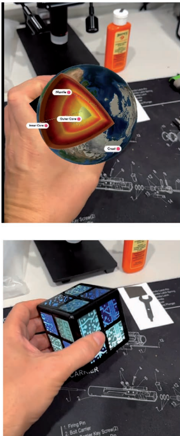
Figure 6. AR GLOBE application running on the WOWCube® system. Screenshots show the augmented reality interface, where the physical rotation of the WOWCube manipulates a virtual globe in real time. The system demonstrates spatial interaction between tangible input and digital content [8].
