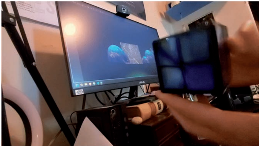
Figure 5. Shows the WOWCube being used as an input device in the Godot game engine to send commands for movement.
