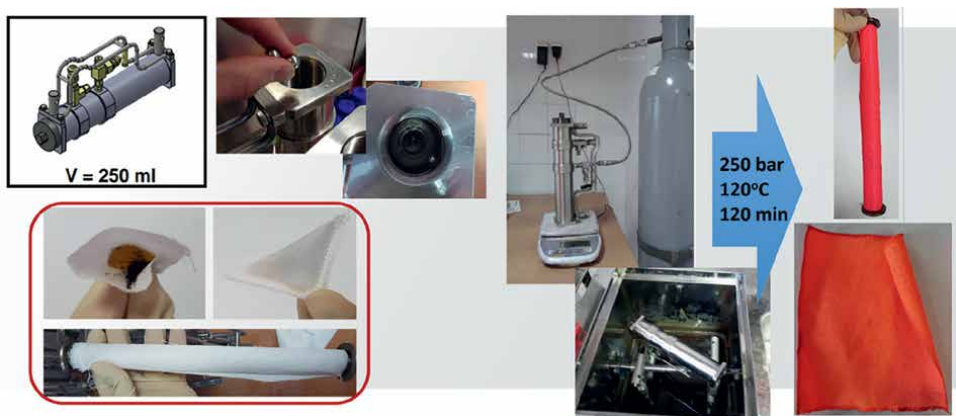
Figure 3. Experimental setup for supercritical CO 2 dyeing [35].
