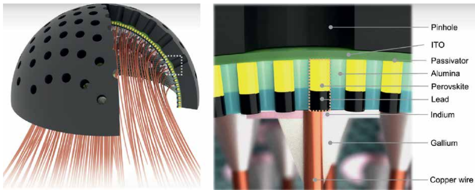
Figure 9. The integrated pinhole compound eye system (left). Exploded view of the PHCE system (right).
