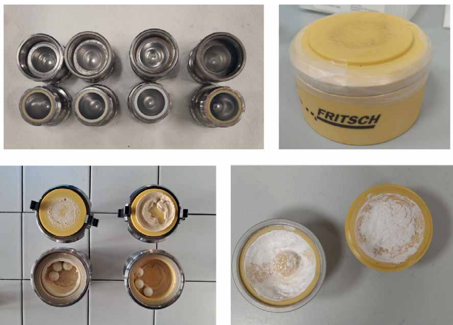
Figure 1. Typical setup employed for a mechanochemical reaction is composed of jars made of either stainless steel or zirconia.
