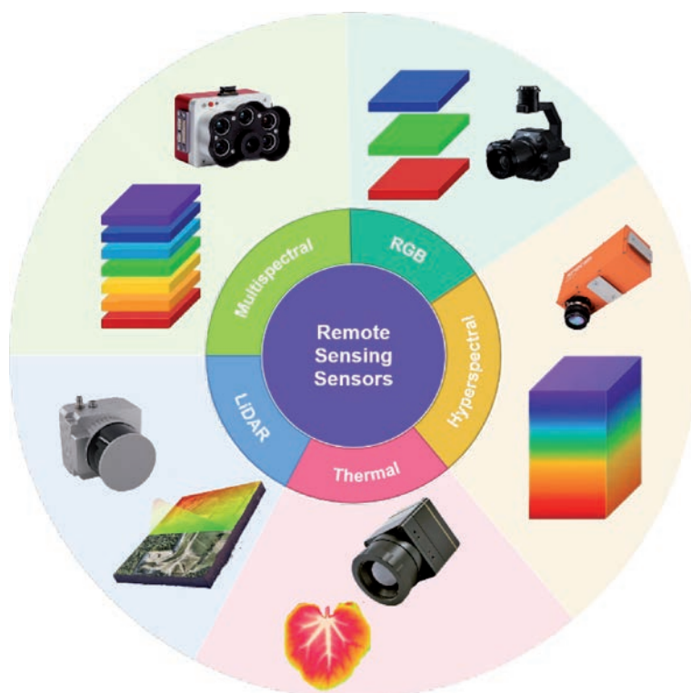
Figure 2. Overview of standard remote sensing sensors based on spectral characteristics: RGB, multispectral, hyperspectral, thermal, and LiDAR. Each category is illustrated with its typical data output and example sensor type, highlighting the diversity of agricultural and environmental monitoring technologies.
