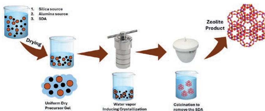
Figure 3. A visual representation of the dry-gel method for zeolite synthesis.
