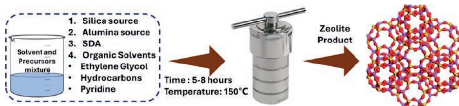
Figure 2. A visual representation of the solvothermal method for zeolite synthesis.
