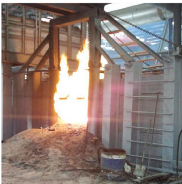
Figure 12. Flames resulting from carbon monoxide generating during tapping.
