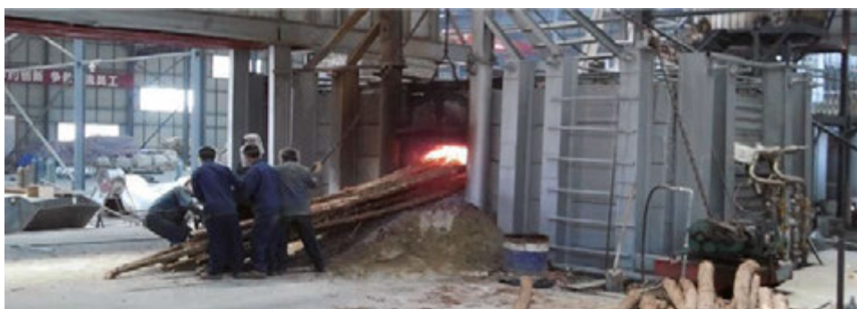
Figure 10. Poling with wood in a 100-ton reverberatory furnace.
