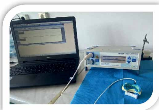
Figure 5. The laser Doppler device, acquisition system and laser probe holder, which ensures the stability of the laser probe and allows repeated measurements.
