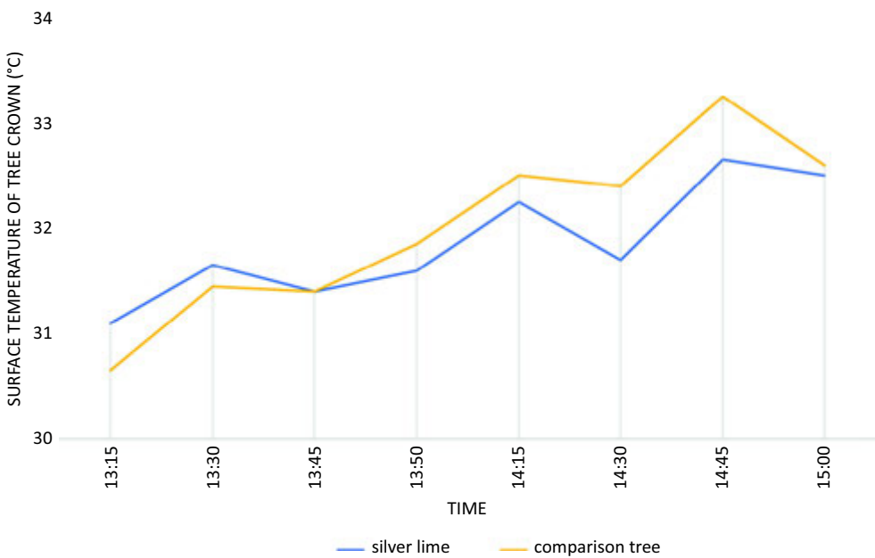
Figure 4. Surface temperature of the canopy of the silver lime tree and a reference tree in Buchenlochstraße on 11 August 2023 [Carl 2024].
