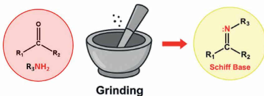
Figure 8. Schematic representation of the solvent-free grinding method (mechanochemical synthesis) for the preparation of Schiff bases.
