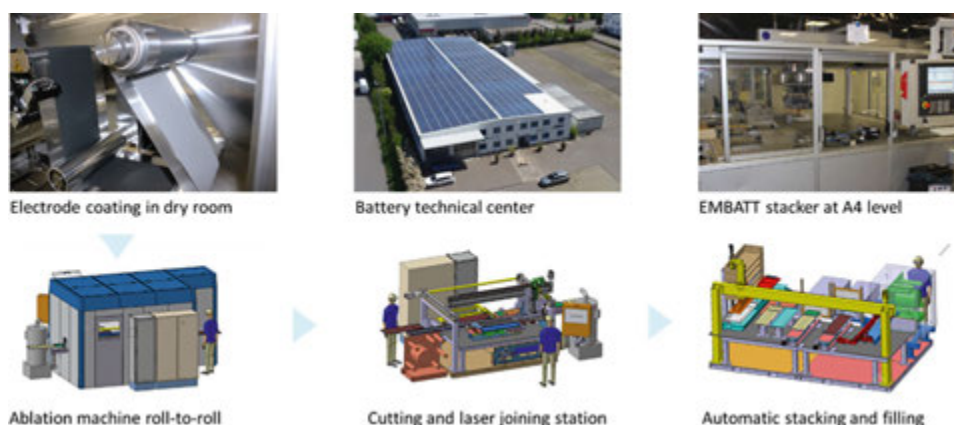
Figure 7. Prototype production line for bipolar cell stack in the EMBATT research project [7].
