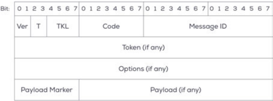
Figure 4. CoAP packet format illustrating the header structure, including version, type, token length, code, message ID, options, and payload, used for lightweight communication in IoT applications.
