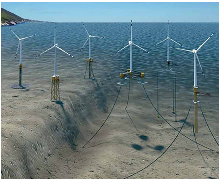
Figure 2. Shallow vs. deep waters wind turbine installations.
