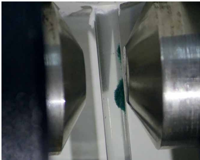
Figure 1. Paramagnetic particles are attached by strong magnetic fields of an electromagnet while immersed in a liquid medium.
