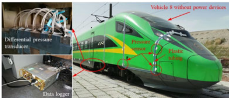
Figure 2. The configuration of full-scale measurement of a HST in China [14].
