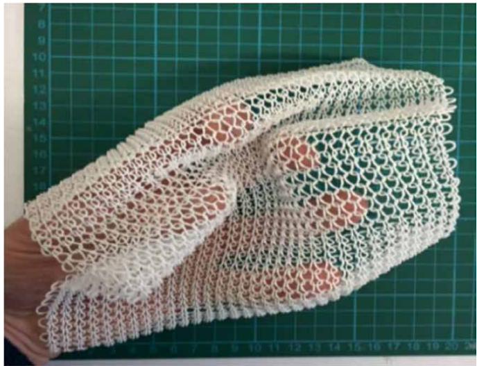
Figure 11. A view of the fabric produced by the 3D printing method, which is similar to the weft knitted fabric [10].
