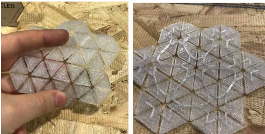
Figure 12. A view of fabric produced with recycled materials by a 3D printer [11].
