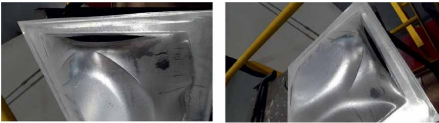
Figure 20. Photos of the formed part of the SPF trial 1.
