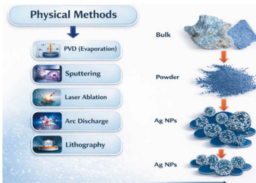
Figure 4. Schematic diagram for physical synthesis of AgNPs.
